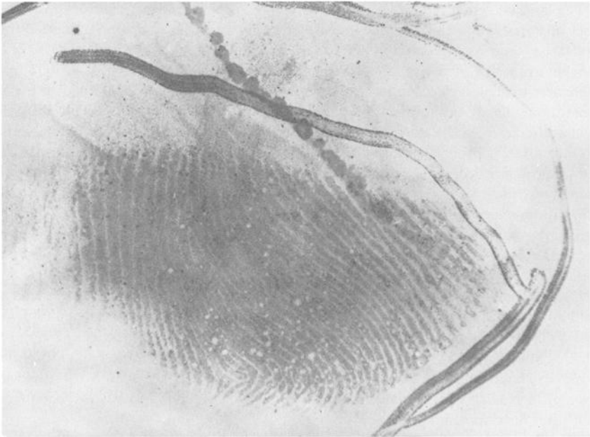
FIG. 2— Latent fingerprint on a sample from Fig. 1, developed by dye laser. This black-and-white print was made from a color slide. The several reproduction steps leading from original slide to printed page cause substantial loss of detail.
